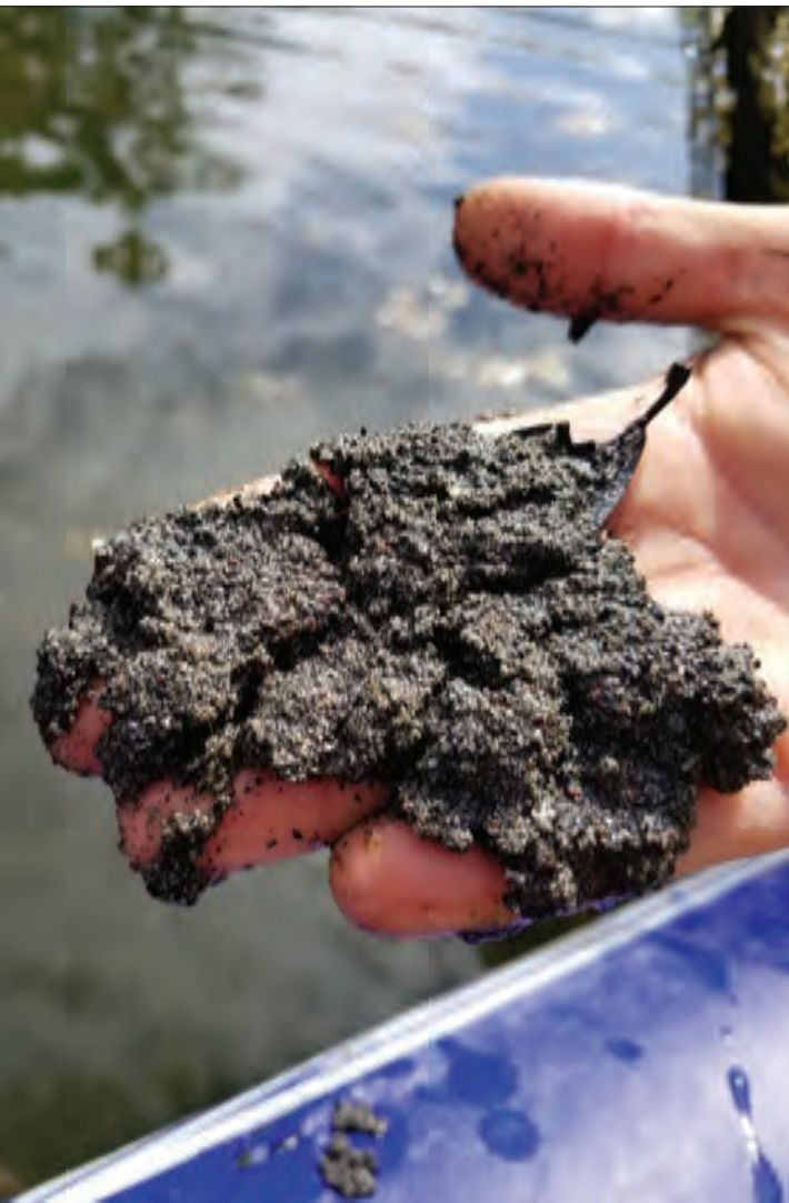
Figure 36. Topsoil and sand were mixed to form a thin-layer cap over contaminated lake sediments. This cap does not support freshwater mussels, although they do occur in adjacent natural substrate.
