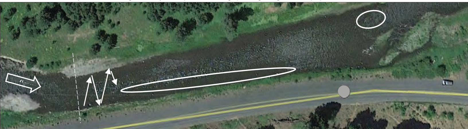
Figure A3.7. Example of a thorough site search that included surveys of upper project boundary (dashed line), diagonal, bank to bank transect lines (arrows), mussel bed areas with >1 mussel/m 2 (white ovals). The initial surveys were conducted with view buckets and identified areas of higher M. falcata density. These areas of higher density will be prioritized during upcoming salvage efforts in preparation of in-channel restoration activities.
