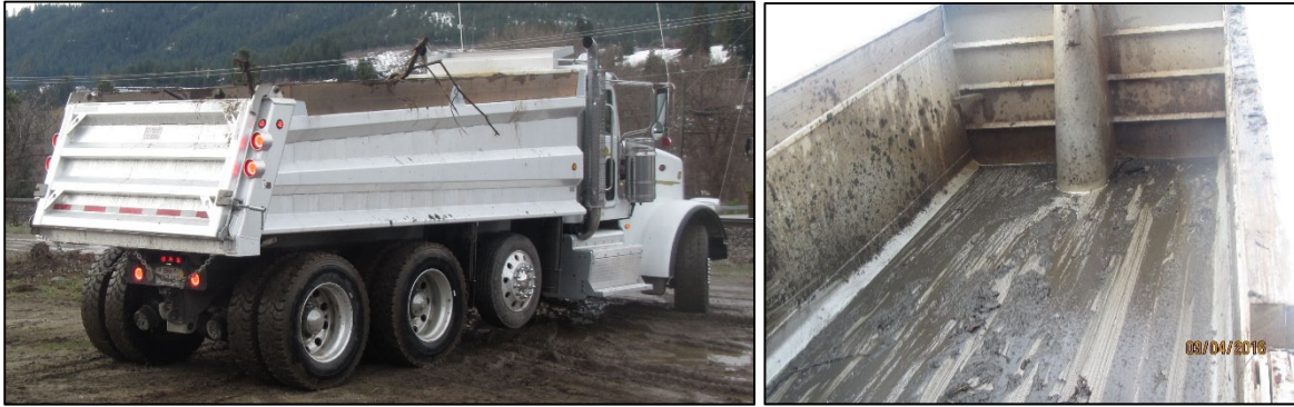
Figure 3. Custom-made waterproof dump truck owned by Wilsonville Concrete Products (Wilsonville, OR). Overview (left photo) and the inside (right photo).
